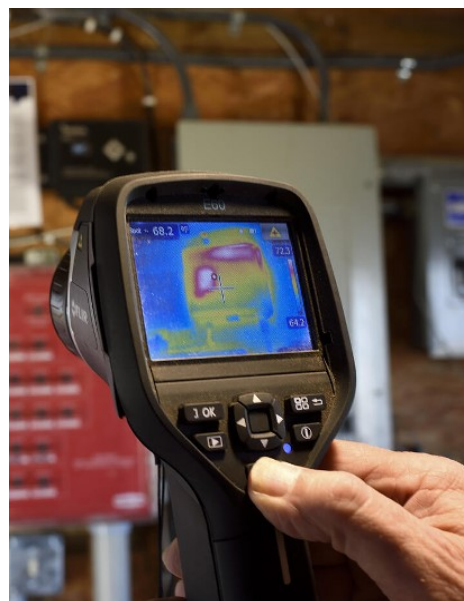
A thermal imaging camera is used to detect hot spots in commercial poultry houses. (Photo by MSU Extension Service/Kevin Hudson) (Editor's Note: Pic-
